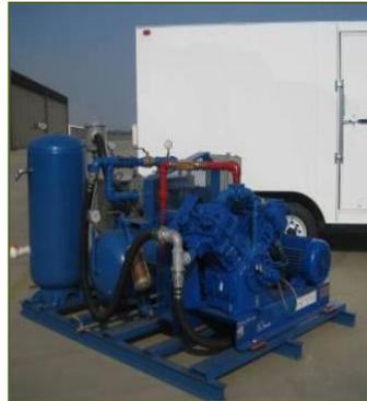
Since late 2009, a cryogenic compression and condensation process has been used to recover hydrocarbons from SVE operations at the **State Road 114 Superfund site** in Levelland, Texas. Over the first seven months of operation, the process brought in project revenue of approximately \$45,000, approximately 70% of the SVE system’s electricity costs.
