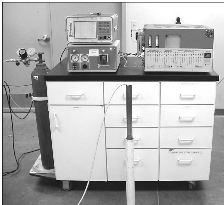
Figure 4.1 The MIP probe is placed in a PVC pipe containing the standard solution.
