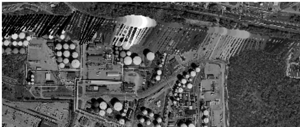
Figure 57. Point leakages from area 2, due to cleaning of a pipeline, see Figure 56. White points correspond to the highest values. (Aerial photo: Copyright Lantmäteriet 2004-11-09. Ur Din Karta och SverigeBilden)
