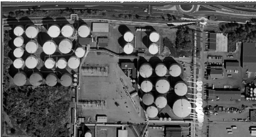
Figure 55. SOF emissions measurements at area 1 showing values around 13 kg/h. White points correspond to the highest values. (Aerial photo: Copyright Lantmäteriet 2004-11-09. Ur Din Karta och SverigeBilden)
