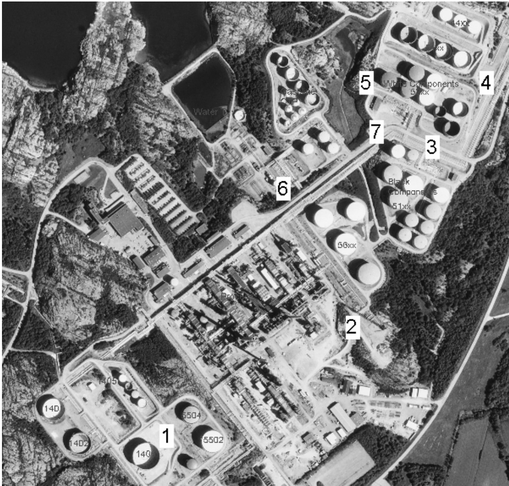
Figure 37. Numbers indicates the positions where samples were taken to retrieve the ratio between aromatic hydrocarbons and alkanes. (Aerial photo: Copyright Lantmäteriet 2004-11-09. Ur Din Karta och SverigeBilden)
