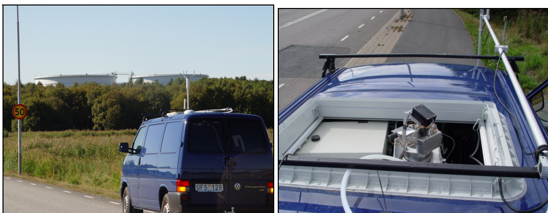
Figure 2. The solar-tracker shown on the right transmits the solar light into the infrared spectrometer independently of the positioning of the car.
