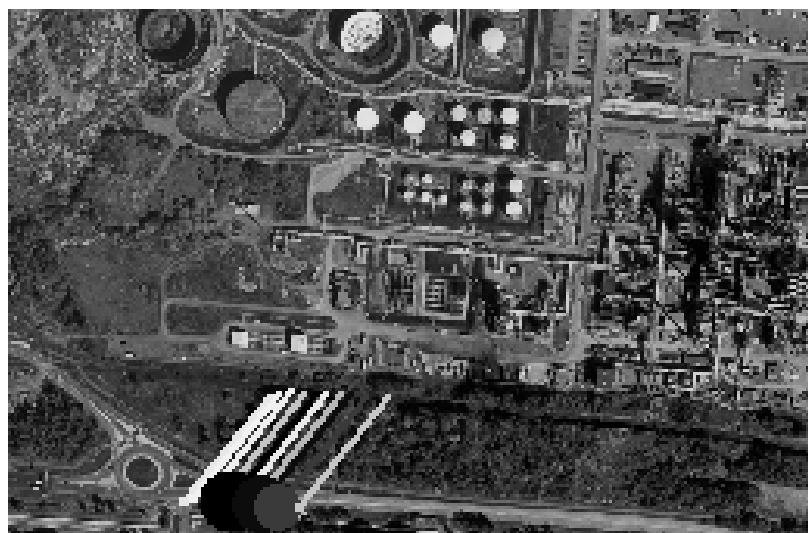
Figure 47. Measurement on the water treatment facility along Oljevågen. Dark points correspond to the highest values. (Aerial photo: Copyright Lantmäteriet 2004-11-09. Ur Din Karta och SverigeBilden)
