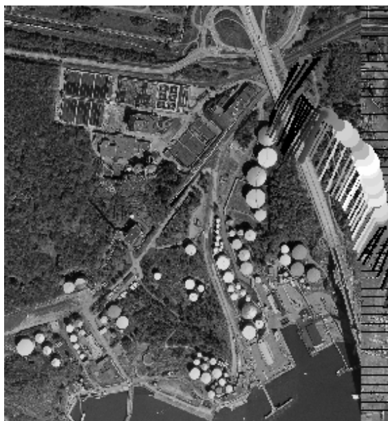
Figure 67. Emission from area 7 measured in 2003 and corresponding to 35 kg/h. White points correspond to the highest values. ( Aerial photo: Copyright Lantmäteriet 2004-11-09. Ur Din Karta och SverigeBilden )
