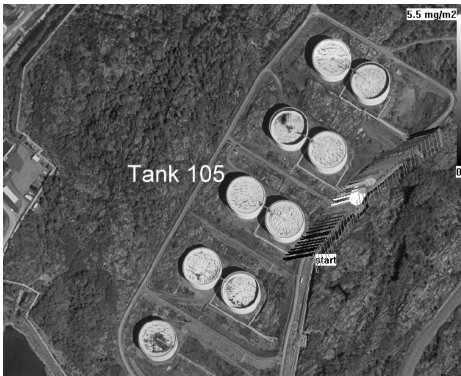
Figure 11. A typical traverse done when the SF 6 gas was emitted on top of tank 105. The broad lines along the traverse points towards the wind direction. (Aerial photo: Copyright Lantmäteriet 2004-11-09. Ur Din Karta och SverigeBildern)
