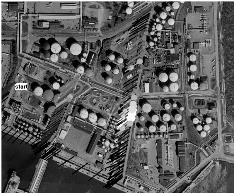
Figure 61. SOF measurement on area 4a and 5a on May 31 2004. Emissions from the whole area correspond to about 26 kg/h. The west part of the area correspond to about 5 kg/h here. The main emission is potentially caused by a previous gasoline leakage along pipelines which occurred in early spring. White points correspond to the highest values (Aerial photo: Copyright Lantmäteriet 2004-11-09. Ur Din Karta och SverigeBilden)
