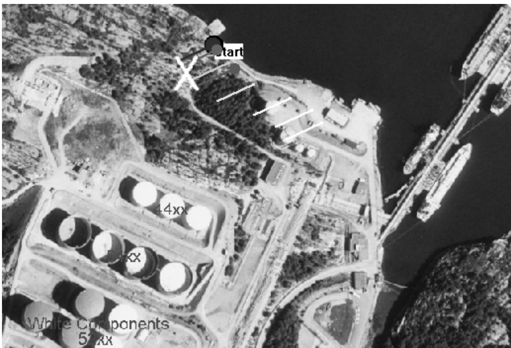
Figure 35. Example of traverse done on the rock cavern exhaust, day 29 July 2004. The position of the rock cavern exhaust is marked with X. Dark points correspond to the highest values ( Aerial photo: Copyright Lantmäteriet 2004-11-09. Ur Din Karta och SverigeBilden )
