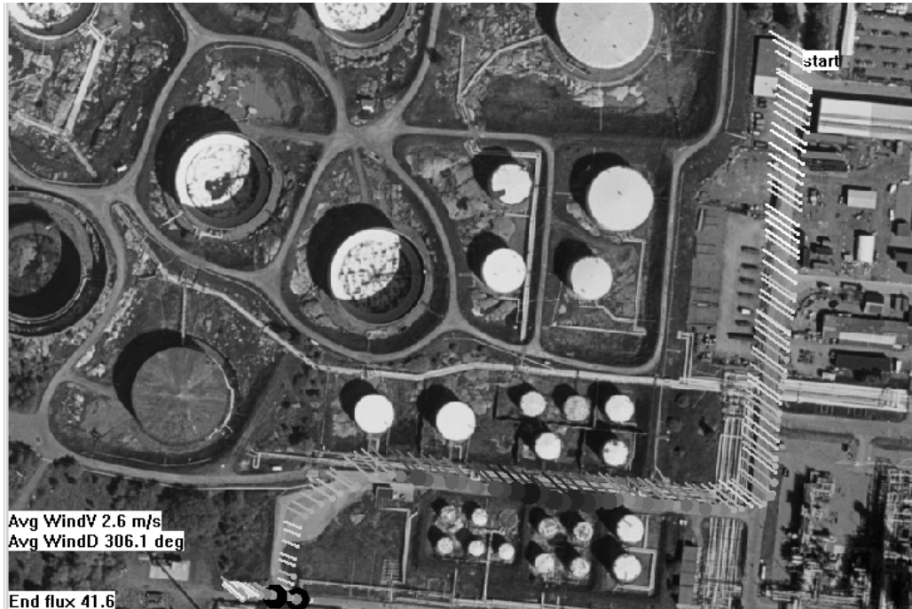
Figure 40. Example of total measurement on the west tank-park, day 29 July 2003. Dark points correspond to the highest values. (Aerial photo: Copyright Lantmäteriet 2004-11-09. Ur Din Karta och SverigeBilden)
