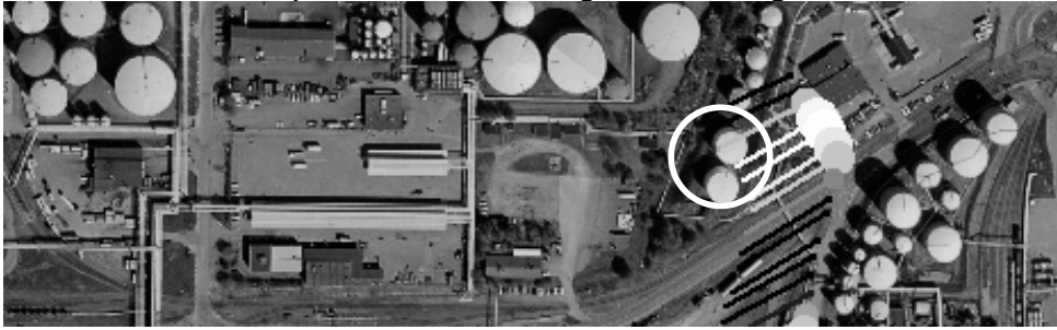
Figure 58. SOF measurements on area 3 on May 31 2004 corresponding to 13 \pm 3 kg/h. The gasoline tanks 101 and 102 are marked by a circle. Here the wind is coming from area 2 where emissions usually are found. White points correspond to the highest values. (Aerial photo: Copyright Lantmäteriet 2004-11-09. Ur Din Karta och SverigeBilden)
