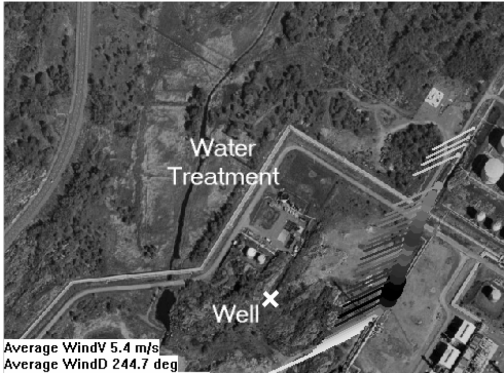
Figure 23. Example of measurement on the water treatment facility day 23-September 2003. Dark points correspond to the highest values. ( Aerial photo: Copyright Lantmäteriet 2004-11-09. Ur Din Karta och SverigeBilden ).
