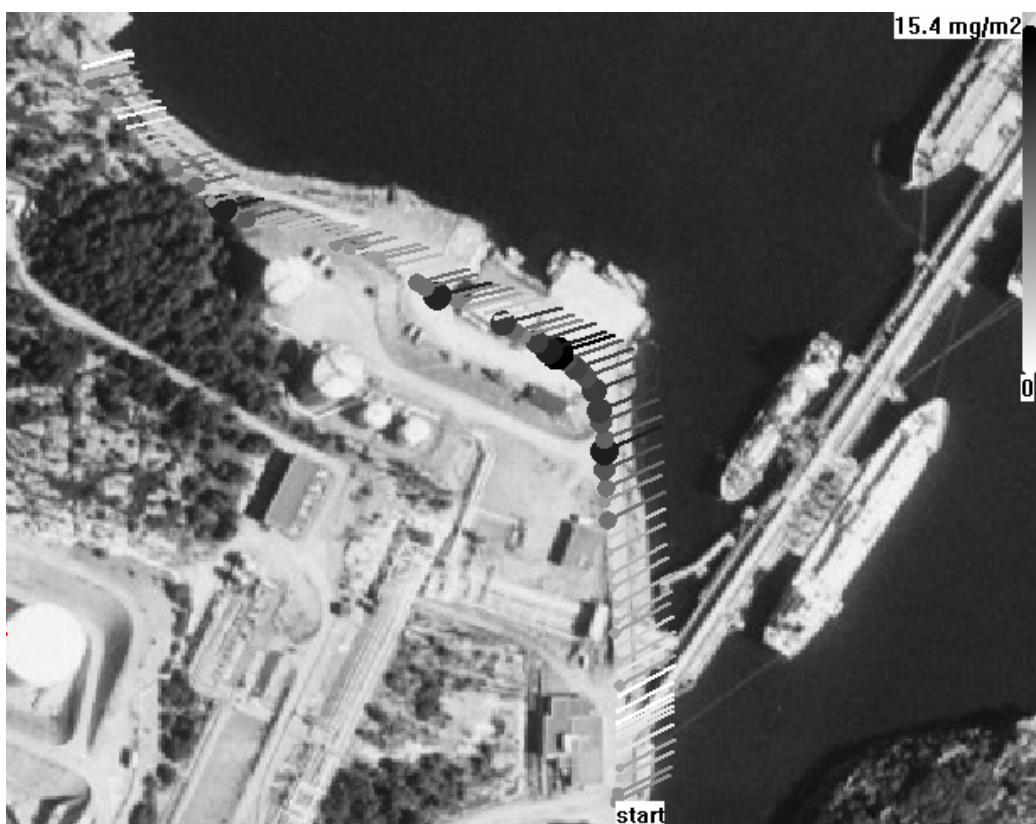
Figure 36. Example of traverse done on the product harbor, day 27 June 2003. Dark points correspond to the highest values. (Aerial photo: Copyright Lantmäteriet 2004-11-09. Ur Din Karta och SverigeBilden)
