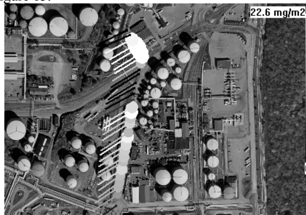
Figure 62. SOF measurement on area 4b on 31-May-2004 corresponding to about 10 kg/h in this measurement. White points correspond to the highest values (Aerial photo: Copyright Lantmäteriet 2004-11-09. Ur Din Karta och SverigeBilden)
