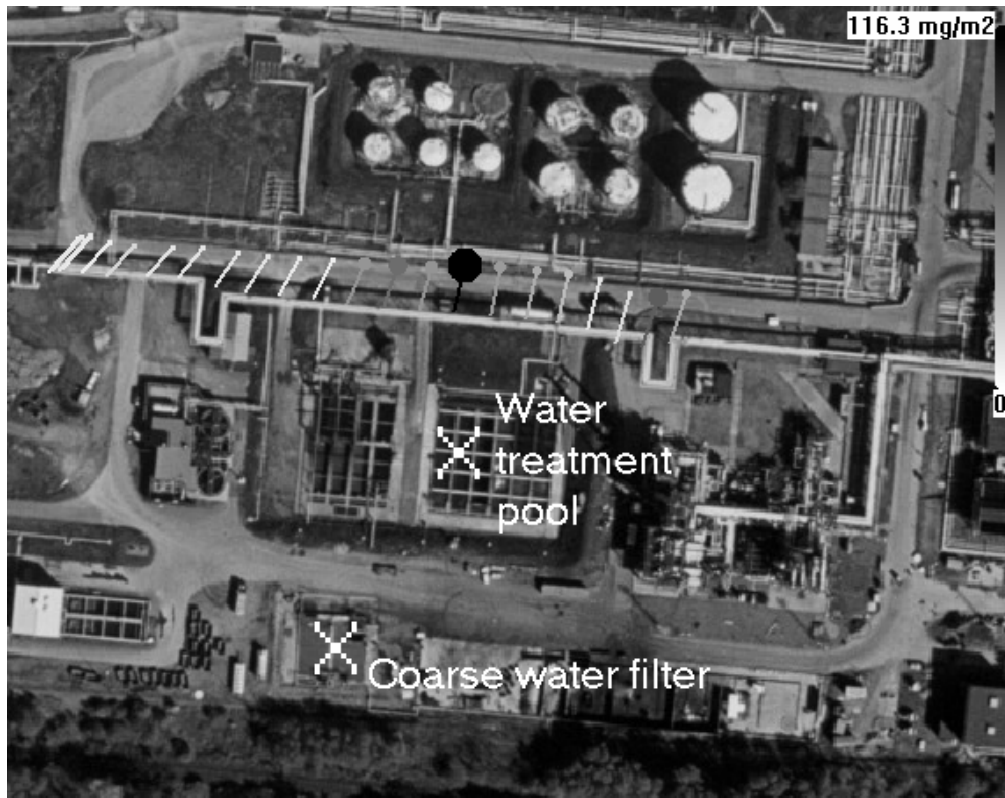
Figure 46. Close measurement on the water treatment facility along the north side. The positions of the water treatment pool and coarse water filter are marked with X. Dark points correspond to the highest values. (Aerial photo: Copyright Lantmäteriet 2004-11-09. Ur Din Karta och SverigeBilden)
