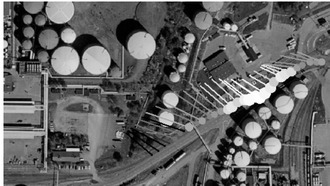
Figure 59. SOF measurements on area 3 on day 15-August-2003 corresponding to 25 kg/h. White points correspond to the highest values (Aerial photo: Copyright Lantmäteriet 2004-11-09. Ur Din Karta och SverigeBilden)
