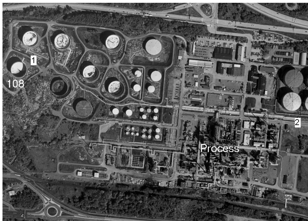
Figure 49. Numbers indicates the positions where samples were taken to retrieve the ratio between aromatic hydrocarbons and alkanes. Dark points correspond to the highest values. (Aerial photo: Copyright Lantmäteriet 2004-11-09. Ur Din Karta och SverigeBilden)
