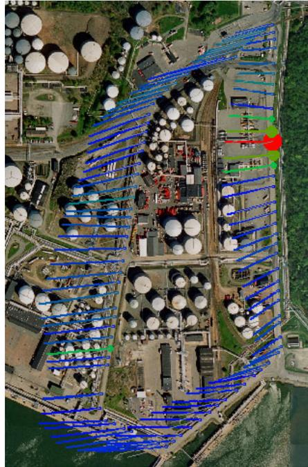
Figure 7. SOF measurements in an oilharbor is shown. Most of the leakages originate from a malfunctioning vapor recovery unit. Red lines indicates points where high values have been measured (maximum value  $160 \text{ mg/m}^2$  here) while blue indicates low values. (Aerial photo: Copyright Lantmäteriet 2004-11-09. Ur Din Karta och SverigeBilden).
