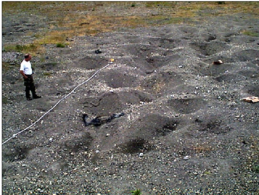
Figure 2. Hand grenade range at Fort Lewis. Tape extends perpendicular from launch area. Note sample jars in rows perpendicular to tape.
