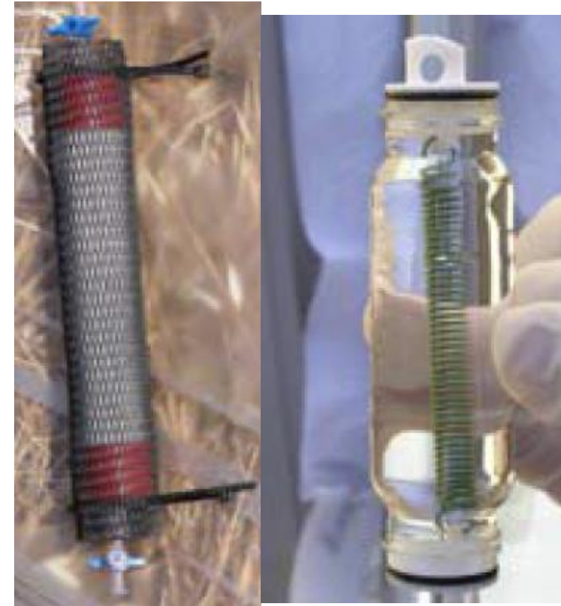
Left: RPP Sampler; Right: Snap Sampler ITRC Technology Overview of Passive Sampler Technologies, March 2006
