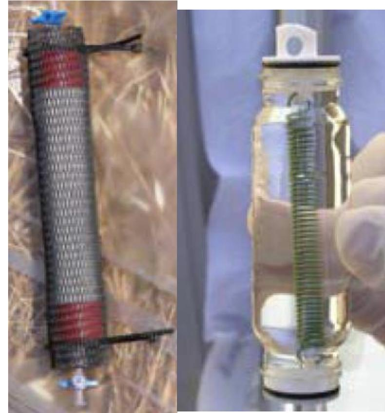
Left: RPP Sampler; Right: Snap Sampler
