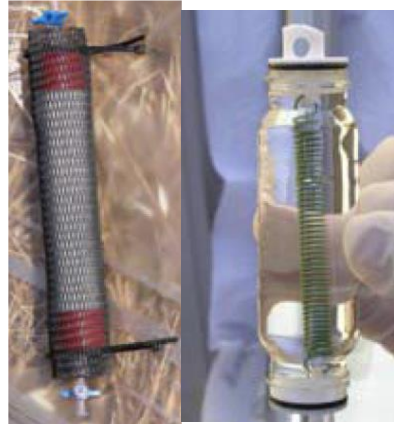
Left: RPP Sampler; Right: Snap Sampler ITRC Technology Overview of Passive Sampler Technologies, March 2006
