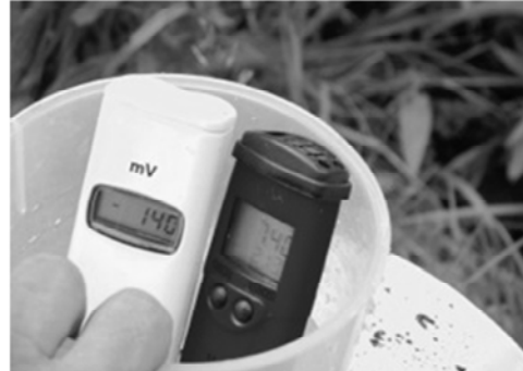
Eh and pH field instruments
