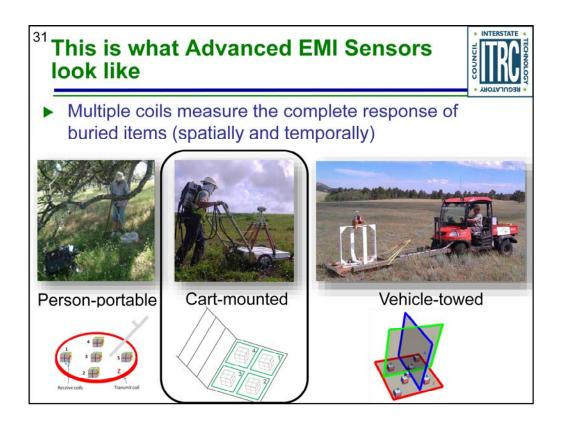
These are prototypes. Standardization of sensors, manuals, procedures are being developed.
