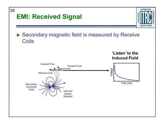
Turn off inducing field and 'listen' to the induced field, which is how we get information about the target
