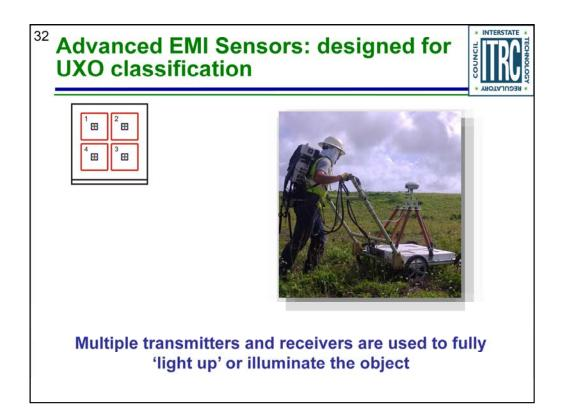
Multi-axis receivers...for a given transmitter, additional information can be obtained by using multiple receivers orientated perpendicularly
