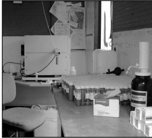
Direct sampling ion trap mass spectrometry (SW846 Method 8265) with mobile lab provides up to 80 soil/groundwater and 60 soil vapor VOC analyses per day
