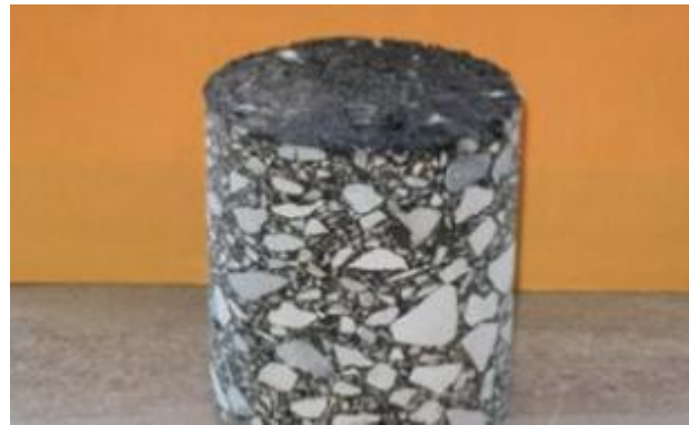
Asphalt concrete with mining waste (chat) making up part of the aggregate mix. MW-1: Figure 4-1
