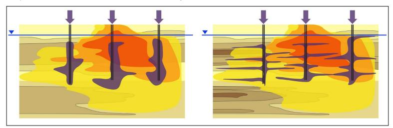
The less heterogeneous case (left) results in delivery of amendment in the vicinity of each of the delivery points.
