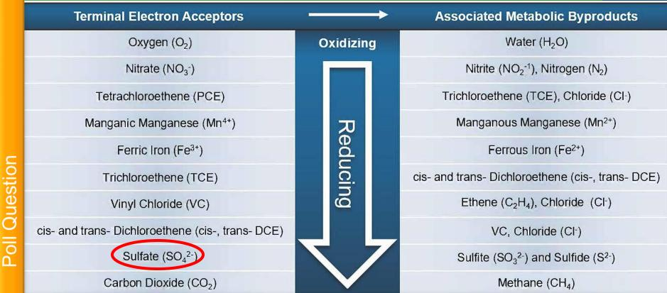
ITRC OIS-ISRP-1 Figure 2-2. Electron acceptors and products in order of reaction preference in progressively reducing groundwater conditions. Select contaminants are included for reference.
