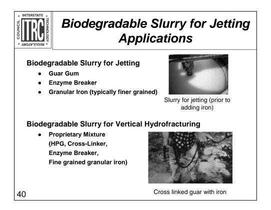
For jetting applications, the biodegradable slurry is used to suspend the granular iron to allow it to be pumped. The enzyme breaker is added prior to injection as the slurry only needs to be viscous for a short time until the granular iron is jetted into place.
