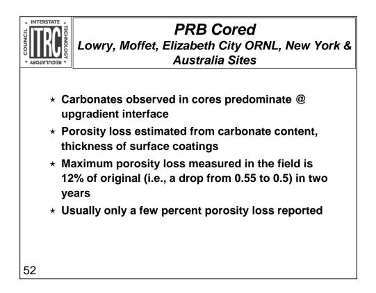
Since recent data suggests this carbonate precipitation will move as a front through the iron as opposed to the initial concept that the carbonate precipitates will continue to form on the upgradient face until the PRB was plugged
