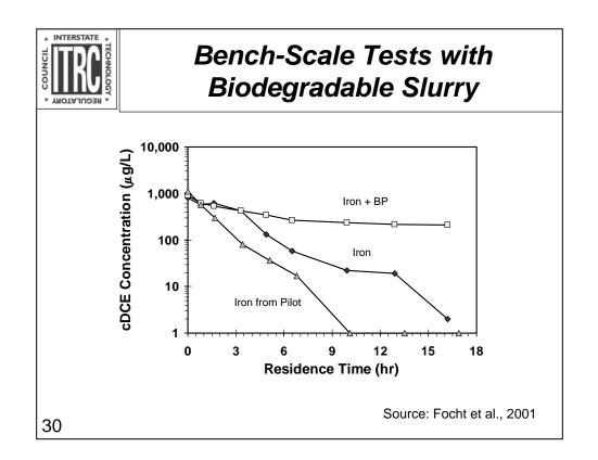
Results from column tests. Residence time is residence time in bench-scale column. "Iron and BP" is an iron column that was saturated with biodegradable slurry then broken with enzyme breaker. "Iron" is an iron column without biodegradable slurry. "Iron from pilot" is iron collected in cores from a pilot installation completed with biodegradable slurry and packed into a laboratory column. All tests were completed at 10 deg. C.
