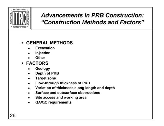
Excavation refers to methods where aquifer material is removed and replaced with the reactive material.
