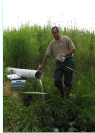
Collecting an effluent sample from BCR discharge point
