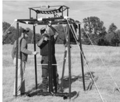
Static test stand to check function of an electromagnetic sensor
