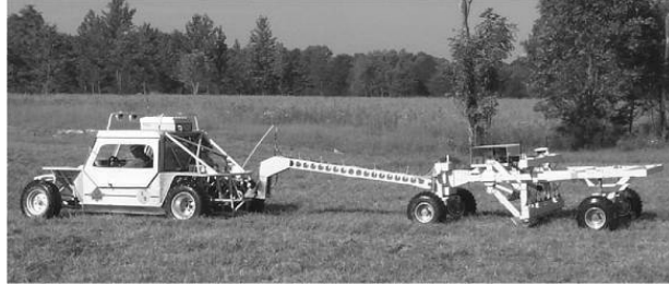
Towed array survey on a GPO test site
