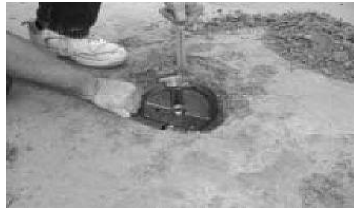
Measuring seed item dip using an inclination protractor
