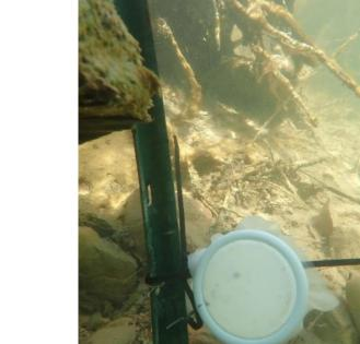
Fig. 4-12. Deployment of a SPATT sampler for cyanotoxins in Zion National Park. Source: Robyn Henderek, used with permission.
