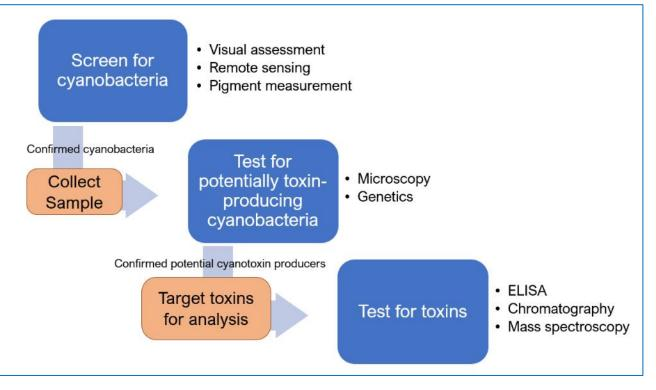
Fig. 4 – 3. Common sequence of monitoring steps used to evaluate risk from HCBs. Source: ITRC, used with permission.
