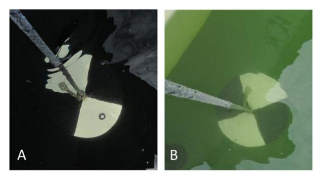
Fig. 4-13. Secchi discs are a common tool to measure water transparency. Source: VT DEC, used with permission.
