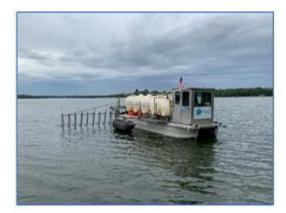
Fig. C – 10. Applying P-binding compounds to a lake. Source Keith Pilgrim, used with permission.
