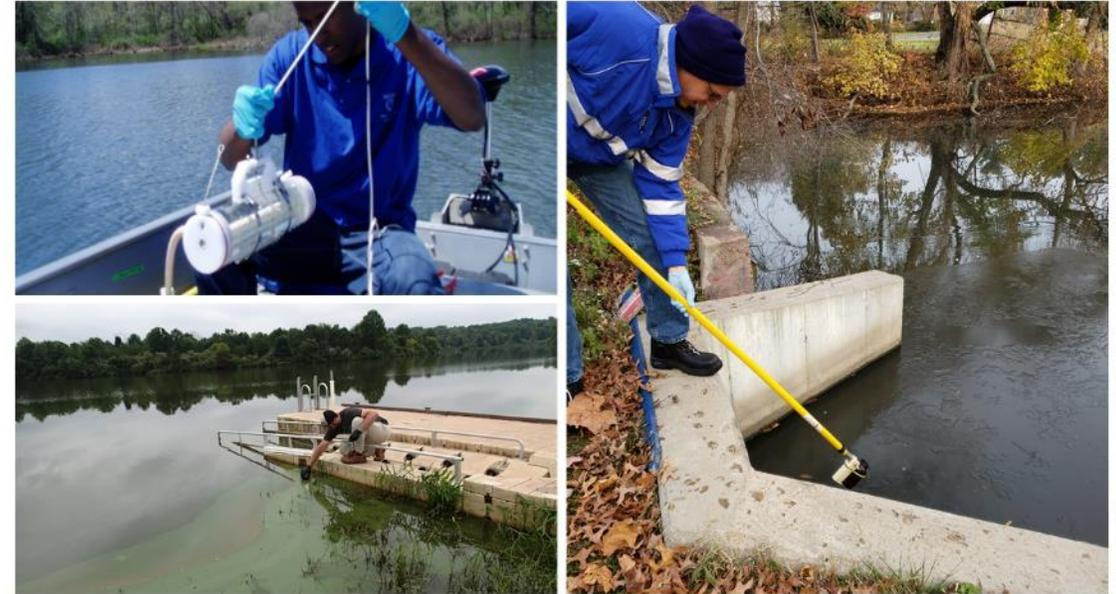
Fig. 4 – 9. Examples of several ways to collect grab samples for cyanobacteria. Source: NJ DEP, used with permission.
