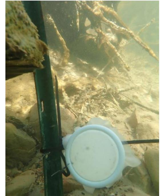
Fig. 4-12. Deployment of a SPATT sampler for cyanotoxins in Zion National Park.
