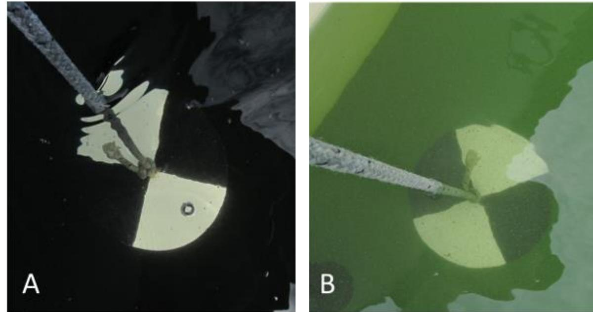
Fig. 4-13. Secchi discs are a common tool to measure water transparency.
