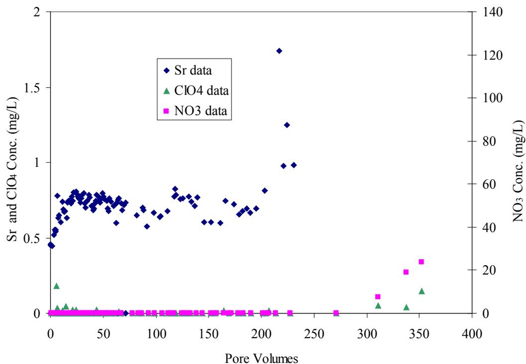
**FIGURE 2. Effluent contaminant concentrations following contact with reactive media in 2-D cell.**
