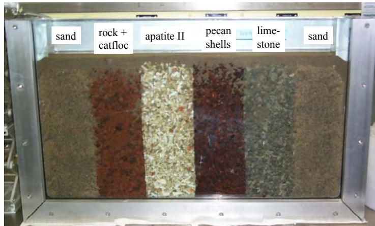
**FIGURE 1. 2-D aquifer cell for treatment of  $^{87}\text{Sr}$ -,  $\text{NO}_3^-$ - and  $\text{ClO}_4^-$ -contaminated groundwater.**
