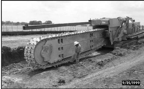
Rock cutter for trenching in weathered limestone bedrock
