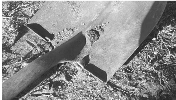
Shovel with NORM-contaminated pipe scale
