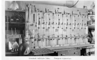
Standard Inducta Tubes - Chlorine Apparatus.
