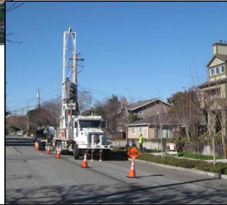
Delineating TCE plume in a residential area near Middlefield-Ellis-Whisman (MEW) Site, California ITRC RMCS-1 Figure 12 (CPEO 2016b)
