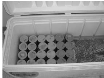
Field curing specimens in a humid atmosphere (water bath).
