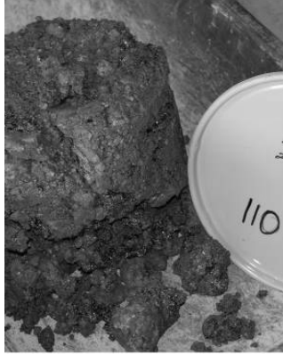
Oily Soil Before S/S
