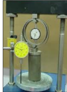
ASTM D1633: UCS for soil-cement cylinders
