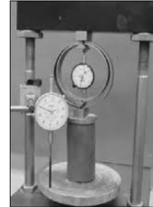
ASTM D1633: UCS for soil-cement cylinders
