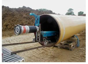
**Note:** The cylindrical source passes through the pipe, and film wrapped around the pipe records the images
