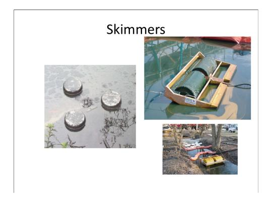
• Image of weir oil skimmer (known as weir skimmers because they rely on oil to flowing into a sump)
