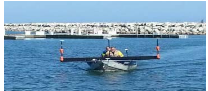
SPAR survey technology outfitted on shallow draft vessel
