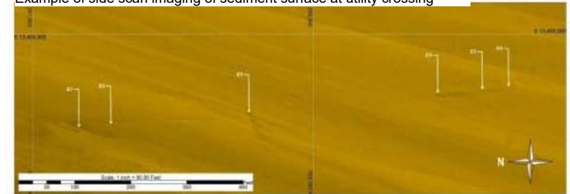
Example of side scan imaging of sediment surface at utility crossing
