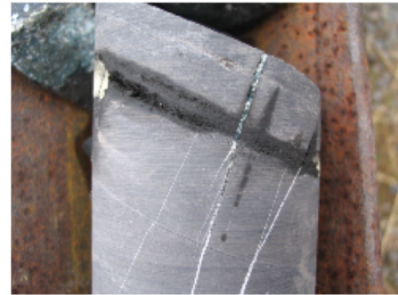
Residual wetting of rock core ( primary/intrinsic rock porosity )
