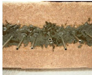
Influent manifold connected to HPLC pump. Typical flow of 0.1 mL/min.
