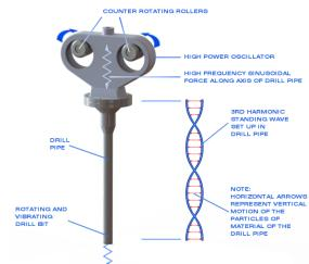
The frequency can be varied to suit operation conditions and is generally between 50 and 160 hertz (cycles per second).
