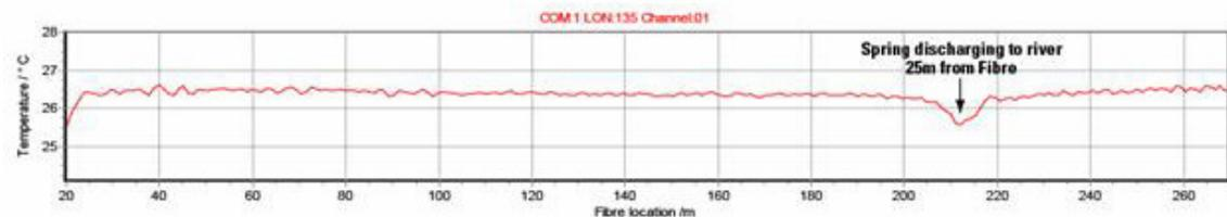
**Figure 2. Sample temperature data from fiber-optic distributed temperature sensor deployed in the Shenandoah River.**
