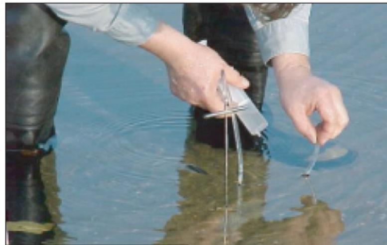
PP27 used as a piezometer/manometer to determine the elevation of ground water relative to surface water
