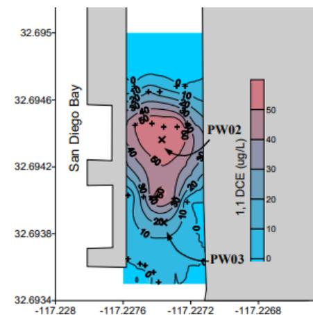
Figure 2-21. 1,1 DCE contour map from porewater samples collected with Trident probe.
