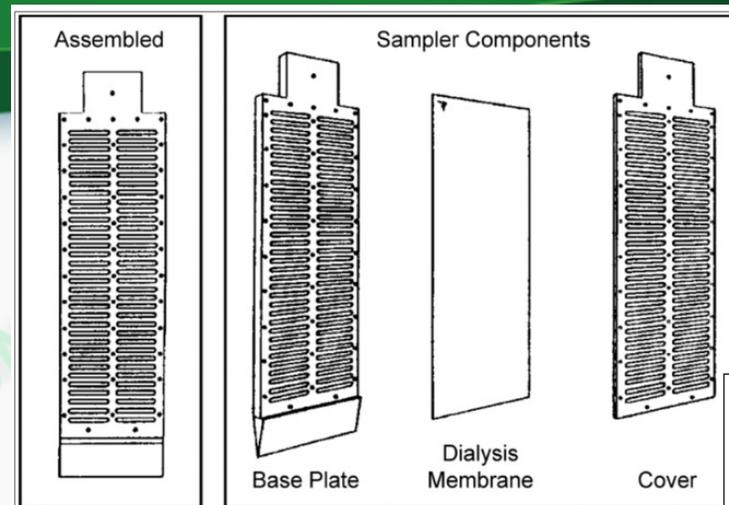
Peeper Plate Device (Source: EPA 2001)
