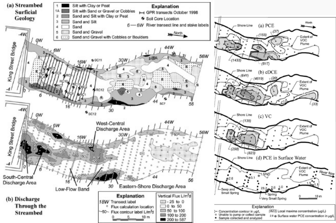
Fig. 3. (a) Map of surficial geology of the streambed and (b) map of vertical water fluxes through the streambed for February 1999.
