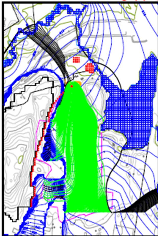
Run 401 - EW-01 Pumping at 50 GPM
