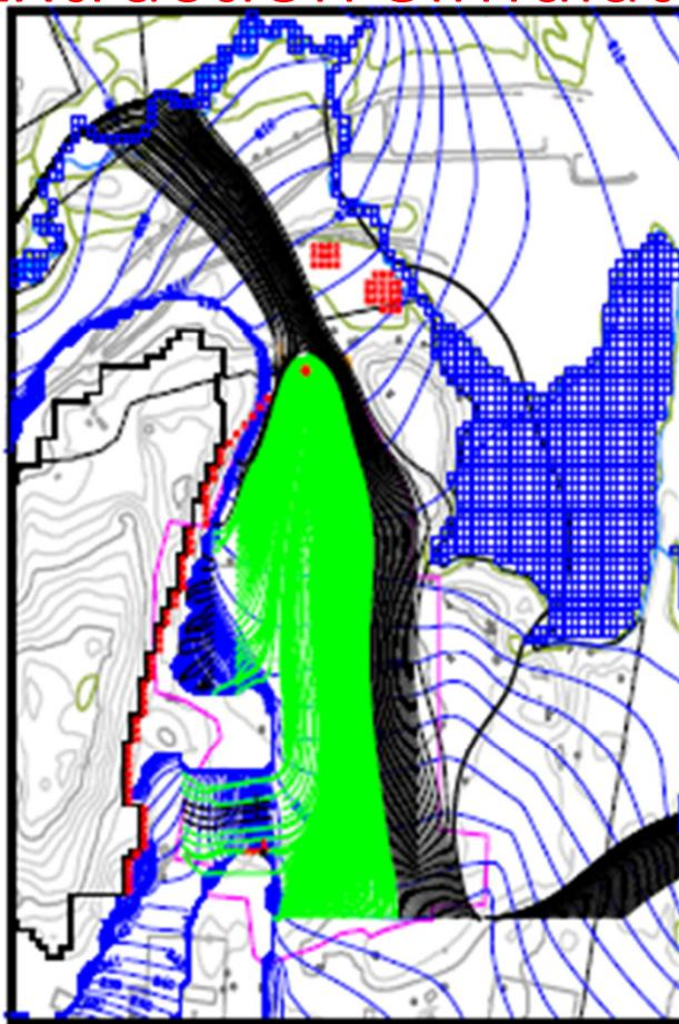
Run 402 - EW-01 Pumping at 40 GPM
