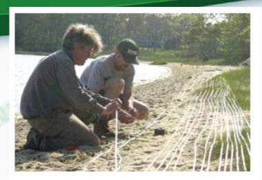
Figure 1. Charles Harvey (MIT) and Fred Day-Lewis (USGS) prepare fiber-optic distributed temperature system for deployment at Waquoit Bay National Estuarine Research Reserve, Massachusetts.
