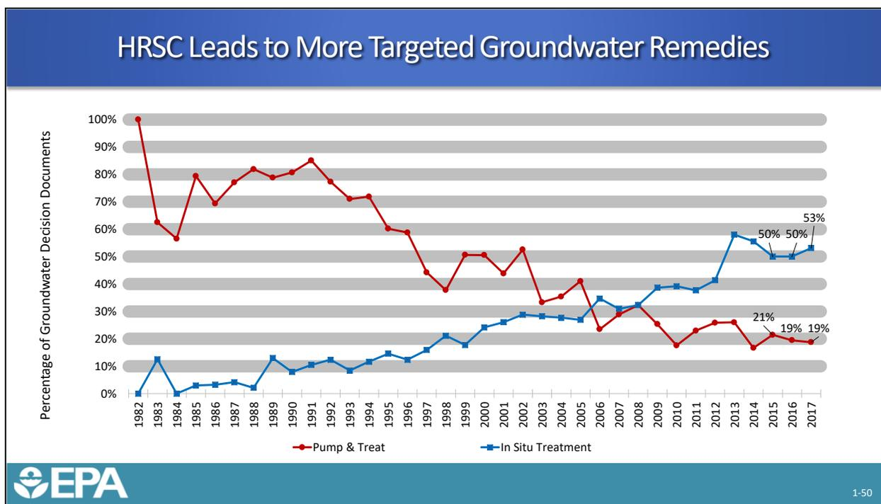
**Main Idea** • *HRSC provides the level of detail necessary to design and implement targeted in situ treatment technologies.*
