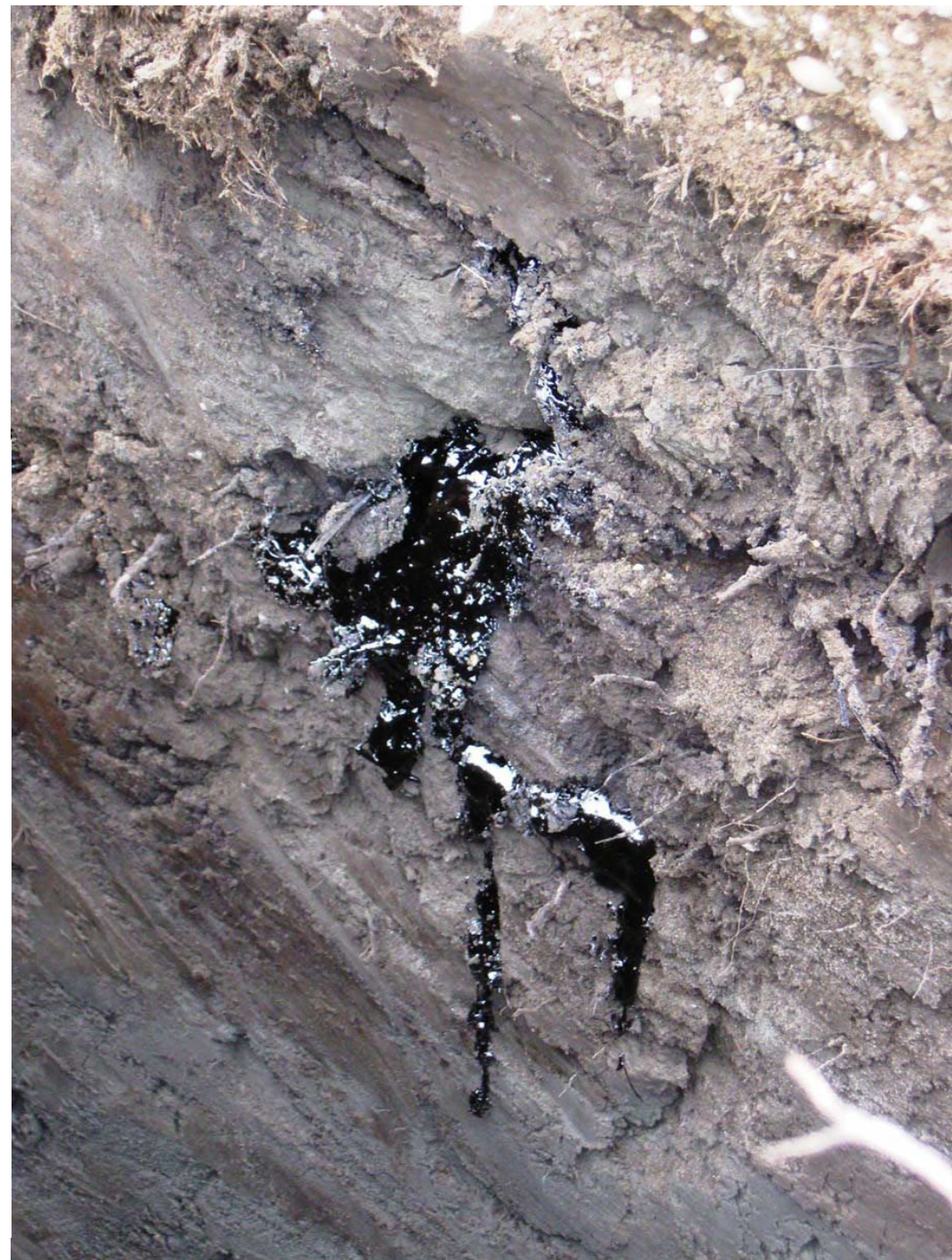
Photograph 30. Boring RI-B7. Discrete tar impacted zone at 153 ft bls. Partially saturated pore spaces of fractured hard limestone unit.
