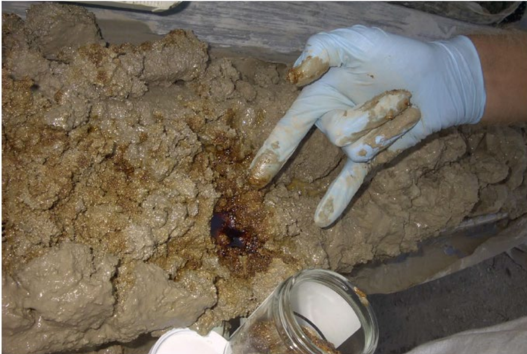
Photograph 30. Boring RI-B7. Discrete tar impacted zone at 153 ft bls. Partially saturated pore spaces of fractured hard limestone unit.
