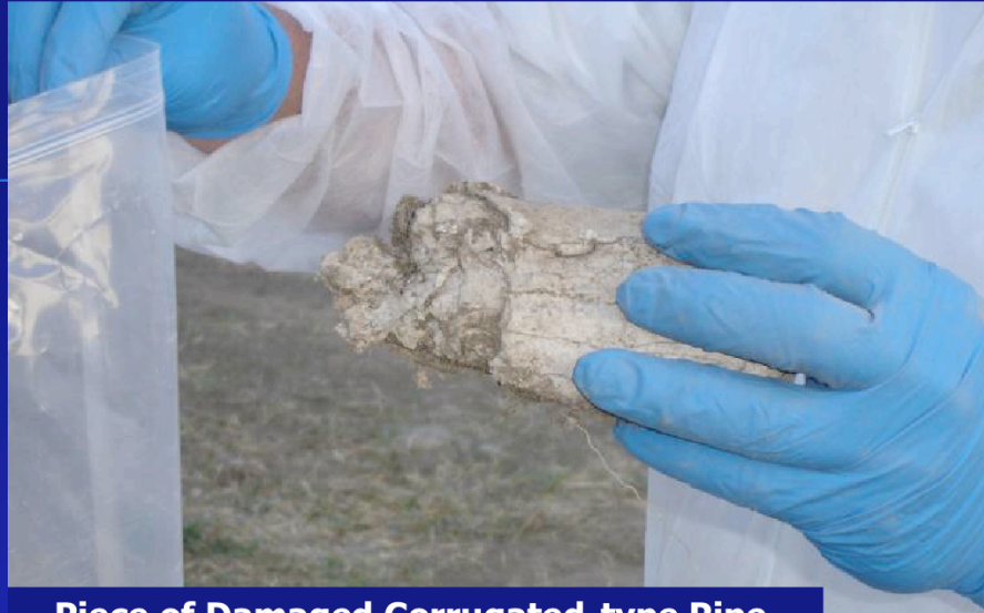
Piece of Damaged Corrugated-type Pipe Insulation Found on Residential Parcel North Ridge Estates
