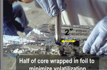
Splitting core tube lengthwise
