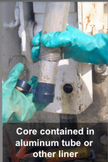
Splitting core tube lengthwise
