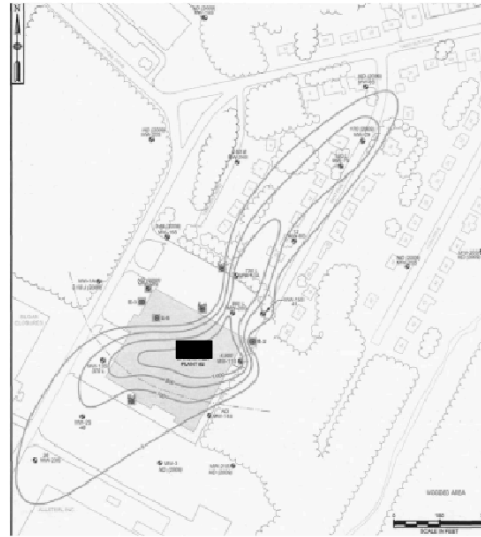
FIGURE X: Institutional controls (ICs) will be necessary to restrict the potable use of groundwater within the contaminated plume, identified above, until groundwater cleanup goals are met.
