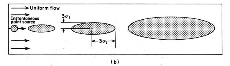
Figure 9.5 Spreading of a tracer in a two-dimensional uniform flow field in an isotropic sand. (a) Continuous tracer feed with step-function initial condition; (b) instantaneous point source.
