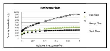
Chemically activated carbonized natural fibers: Demonstration of high adsorption based on pore size and morphology of flax, sisal and hemp fibers
