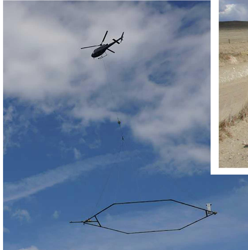
Helicopter towing a geophysical device as part of an electromagnetic and magnetic survey to collect TDEM data ( USGS )
