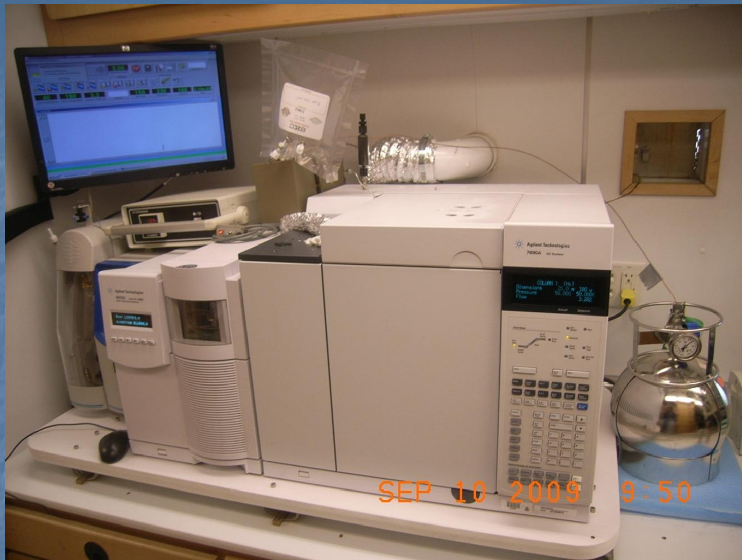
Gas Chromatograph/Mass Spectrometer with Loop Injector for Analysis of Volatiles Compounds Collected in Tedlar Bags
