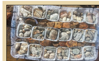
Ranville's team places the clean river rocks (shown here) in a contaminated stream at the North Fork Clear Creek Superfund site to study rates of metal deposition in experimental plots. (Photo courtesy of James Ranville)
