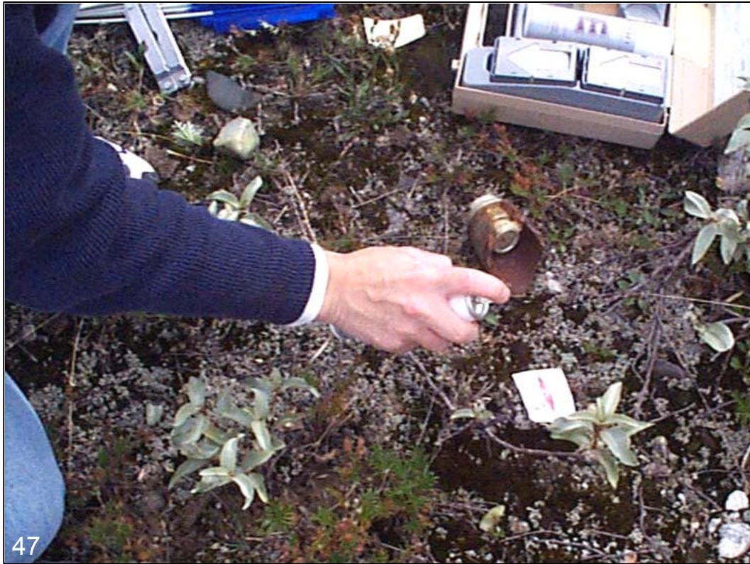
Sampling a piece of partially detonated ordnance for residual explosive. Color shows explosives present.
