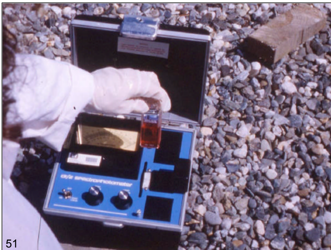
51 Closer view of spectrophotometer and reddish colored solution that forms after addition of reagents to soil extract when TNT is present.
