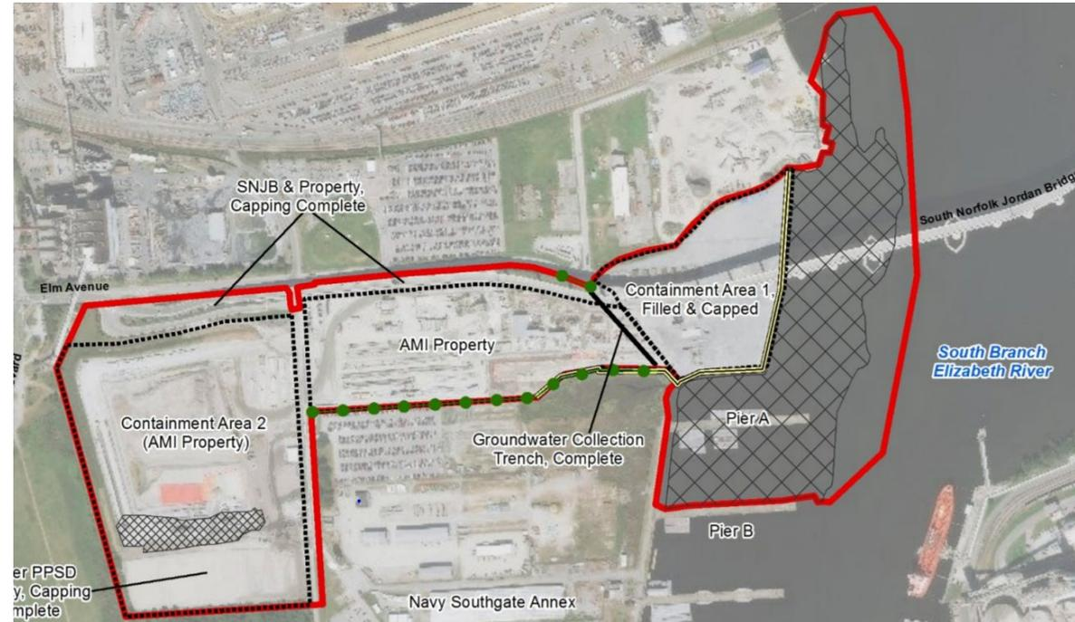
Detailed site map (based on Esri, DigitalGlobe, GeoEye, Earthstar Geographics, CNES/Airbus DS, USDA, USGS, AeroGRID, IGN, the GIS user community, and 2018 remedial design): site boundary (red), sheet pile wall (yellow), planted tree line (green)
