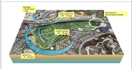
**Note:** Current LTP has a design capacity of 75K gpd, with a possible de-bottleneck capacity of 150K gpd
