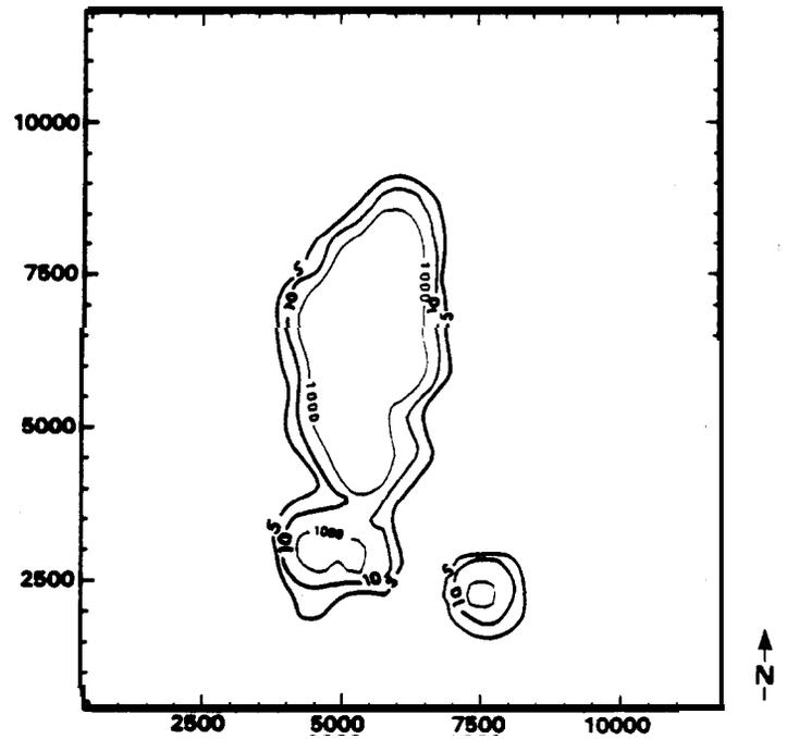
Figure 10.3 Contour Map of the Probability in Percent of a False Positive in the Remedial Action Areas and the 1,000 ppm Contour Line
