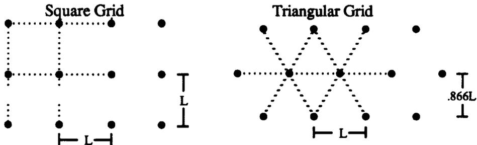
The size of the sample area must be determined in order to calculate the distance,  $L$ , between the sampling locations in the systematic grid. The area can be measured on a map using a planimeter. The units of the area measurement (such as square feet, hectares, square meters) should be recorded.
