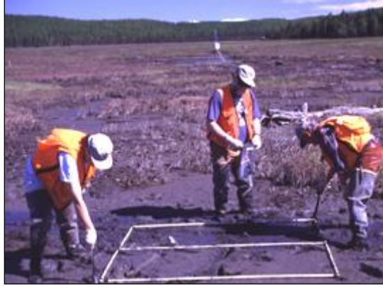
Figure A1-2. Sampling for white phosphorus in sediment using a 1.82-m square quadrat.
